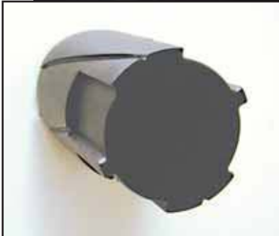
The laser-guided launcher (above) discharges a tagging projectile (left). The tag adheres to the suspect vehicle and transmits its GPS coordinates to a computer server.
