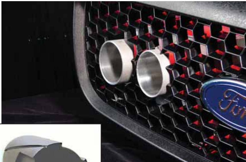
The laser-guided launcher (above) discharges a tagging projectile (left). The tag adheres to the suspect vehicle and transmits its GPS coordinates to a computer server.
